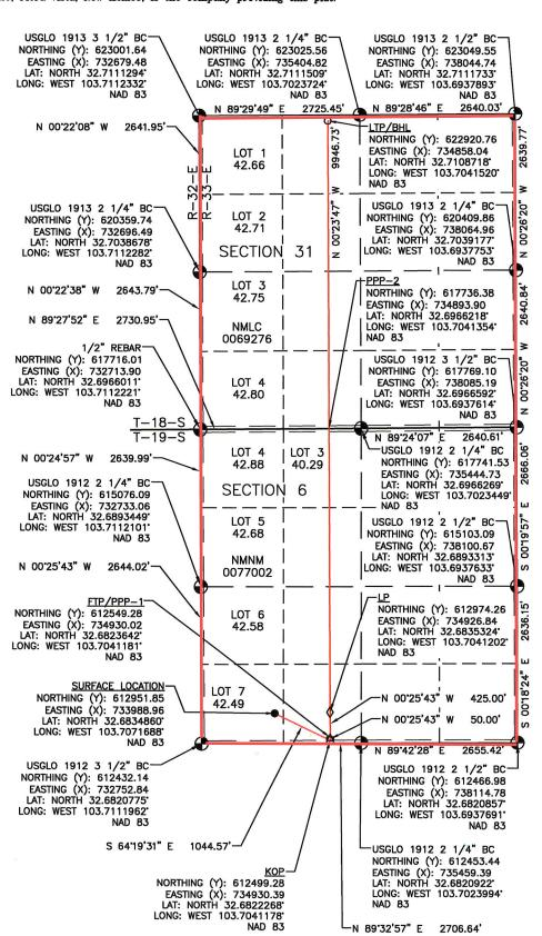
NOTE: BEARINGS AND DISTANCES SHOWN ARE REFERENCED TO THE NEW MEXICO COORDINATE SYSTEM, EAST ZONE, NAD 83, UNLESS OTHERWISE NOTED
