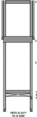
3. Perf @ 100'. Pressure test. Circulate 45 sx cmt to surface.
