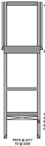
4. Perf @ 100'. Pressure test, good circulation. Circ 45 sx cmt to surf.
