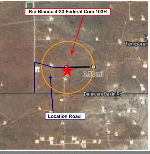
Assumed 100 ppm ROE = 3000' (Radius of Exposure) 100 ppm H2S concentration shall trigger activation of this plan.
