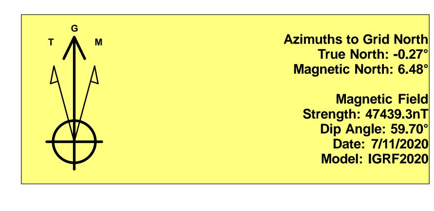
To convert a Magnetic Direction to a Grid Direction, Add 6.48° To convert a Magnetic Direction to a True Direction, Add 6.75° East To convert a True Direction to a Grid Direction, Subtract 0.27°
