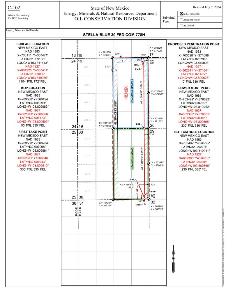
Released on the New Mexico State Plane Coordinate System, East Zone, NAD 83-2011 (EPOCH 2010) iramework, as derived by OPUS Solution. The elevations shown hereon are based on NAVD 88.
