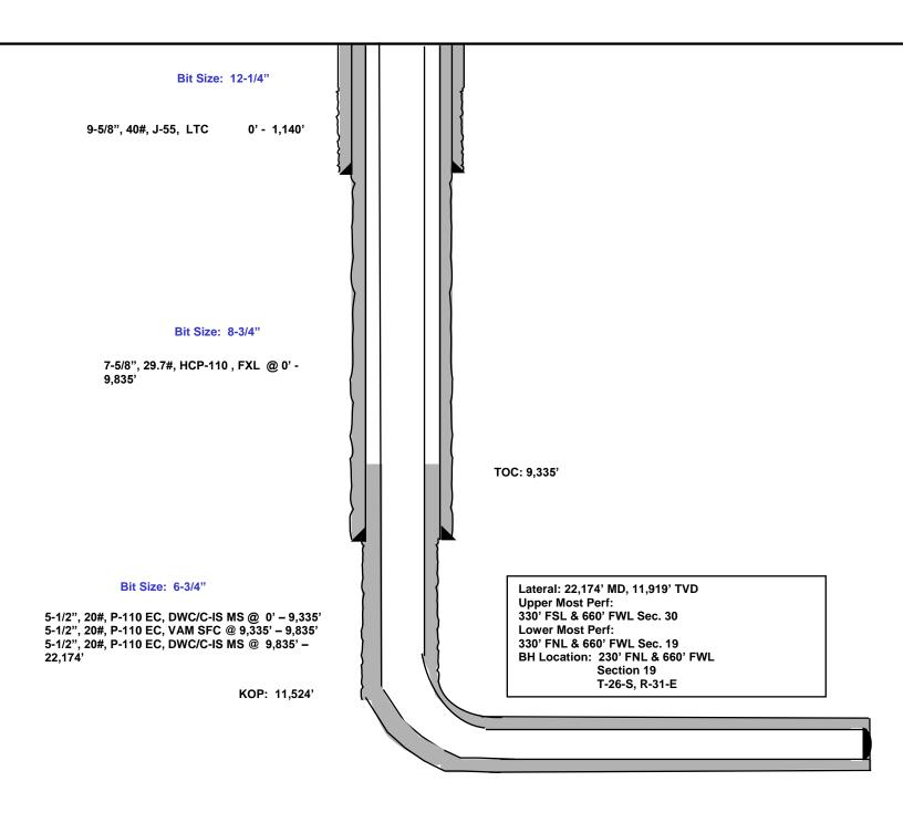
883' FSL 822' FWL Section 30 T-26-S, R-31-E Proposed Wellbore Design B KB: 3,095' GL: 3,070'
