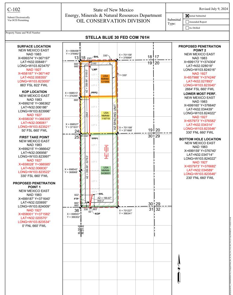
Release Bearings angling to /202 distances shown hereon are based on the New Mexico State Plane Coordinate System, East Zone, NAD 83-2011 (EPOCH 2010) framework, as derived by OPUS Solution. The elevations shown hereon are based on NAVD 88.
