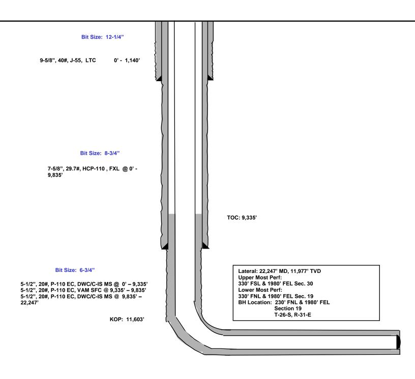
965' FSL 2259' FEL Section 30 T-26-S, R-31-E Proposed Wellbore Design B KB: 3,138' GL: 3,113'
