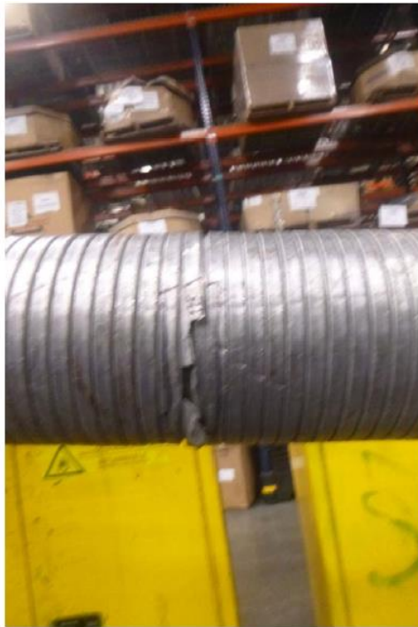
Photo: Damaged armor 11ft 0in. from EF1
