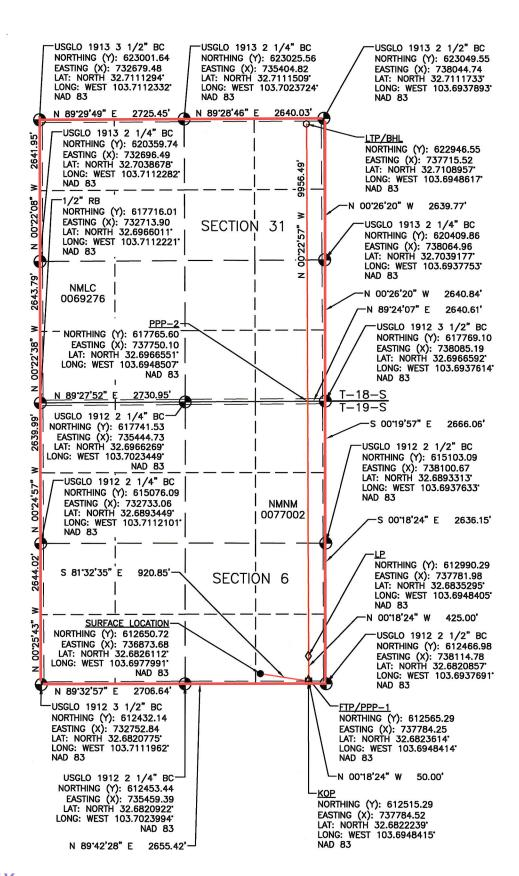
NOTE: BEARINGS AND DISTANCES SHOWN ARE REFERENCED TO THE NEW MEXICO COORDINATE SYSTEM, EAST ZONE, NAD 83, UNLESS OTHERWISE NOTED
