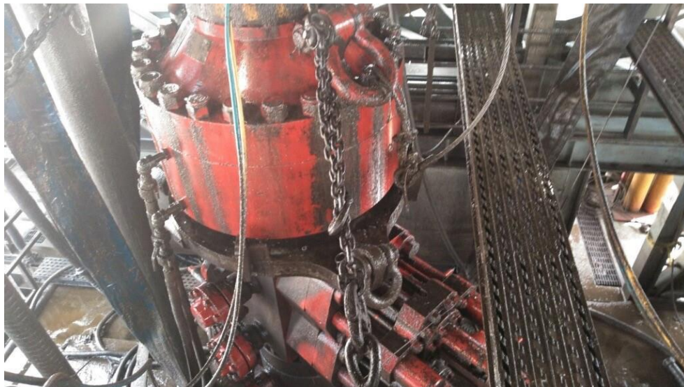
Figure 1: Winch System attached to BOP Stack
