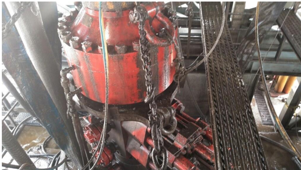
Figure 1: Winch System attached to BOP Stack
