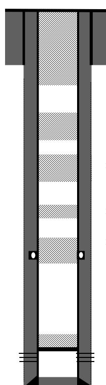
8-5/8" J-55 24# casing @ 201'. Cemented with 135 sks Cement. Circulated 1 bbl cement to surface.
