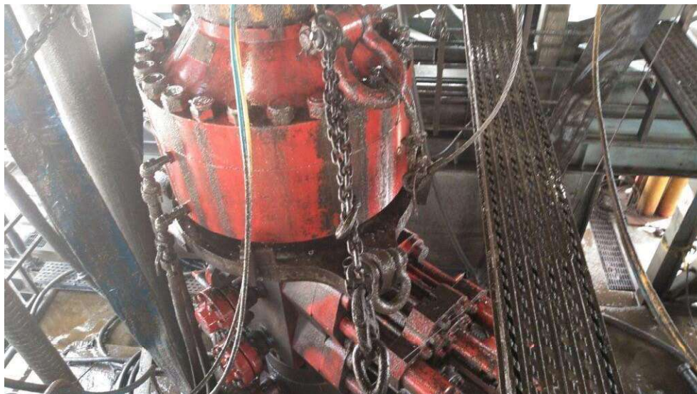
Figure 1: Winch System attached to BOP Stack
