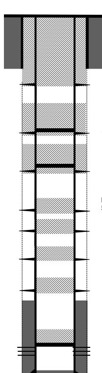
$10\mbox{-}3/4\mbox{''}$  H-40 32.75# casing @ 396'. Cemented with 400 sks.
