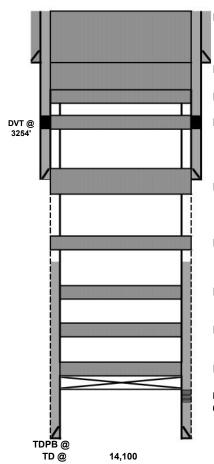
Plug #9: Perf'd @ 500'. Sqz'd 150 sxs class C cmt @ 500' to surface. Tagged TOC @ 45' inside 13 3/8 X 9 5/8 and tagged TOC @ 15' inside 5 1/2". Topped off well with 45
