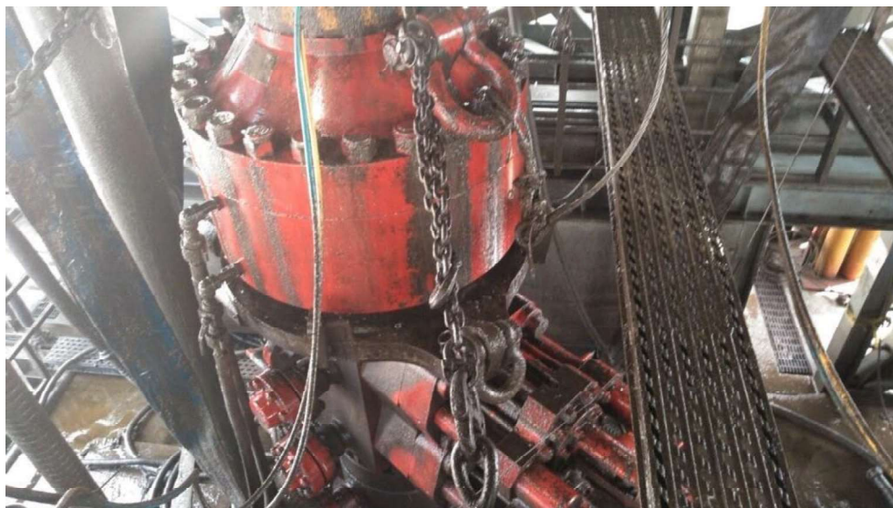
Figure 1: Winch System attached to BOP Stack
