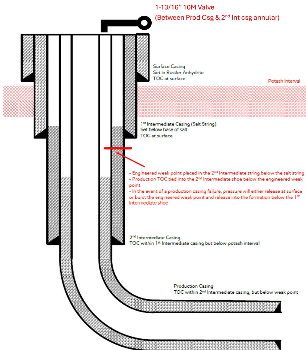
[Figure F] 4 String – 2<sup>nd</sup> Intermediate casing engineered weak point
