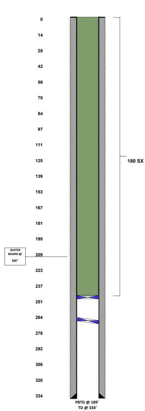
PLUG #1 5/2/25 SET CIBP @ 250' & SPOT/FILL UP W/ 180 SX CLASS " C" CMT TO SURF. RDMO P&A RIG, CUT OFF WH, INSTALL DRY HOLE MARKER, CLEAN LOCATION. TURN OVER TO RECLAMATION DEPT. **P&A COMPLETE.**
