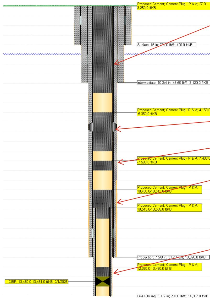
Spot Class C cement from 3,220' to surface. 290 sxs Class C
