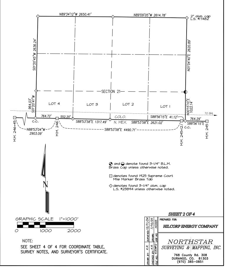
HIILCORP ENERGY COMPANY: ALLISON UNIT #630H SURFACE LOCATION: 538' FNL & 1560' FWL SECTION 12, T-32-N, R-7-W, N.M.P.M., SAN JUAN COUNTY, NEW MEXICO. ELEVATION: 6352' BOTTOM HOLE LOCATION: 201' FSL, 522' FBL
