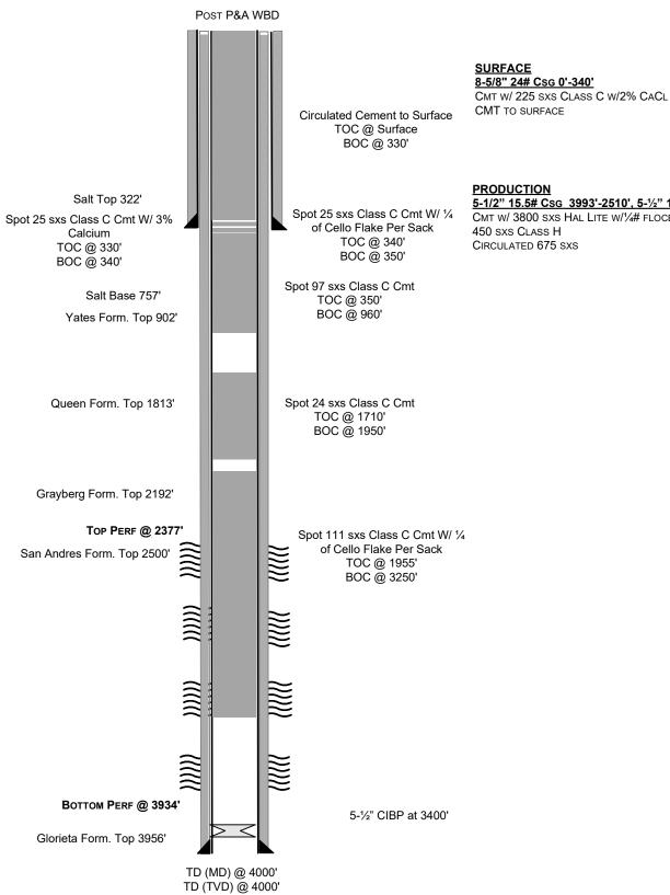
**EVENT LOG** 1/3/1983- SPUDDED 1/13/1983- TD REACHED 2/11/1983-COMPLETED WELL 2665-3230 2/1983- ADDED PERFS 3442-3934, DETERMINED UNPRODUCTIVE, PLACED CIBP AT 3400' 6/1983- ADDED PERFS 2377-2498
