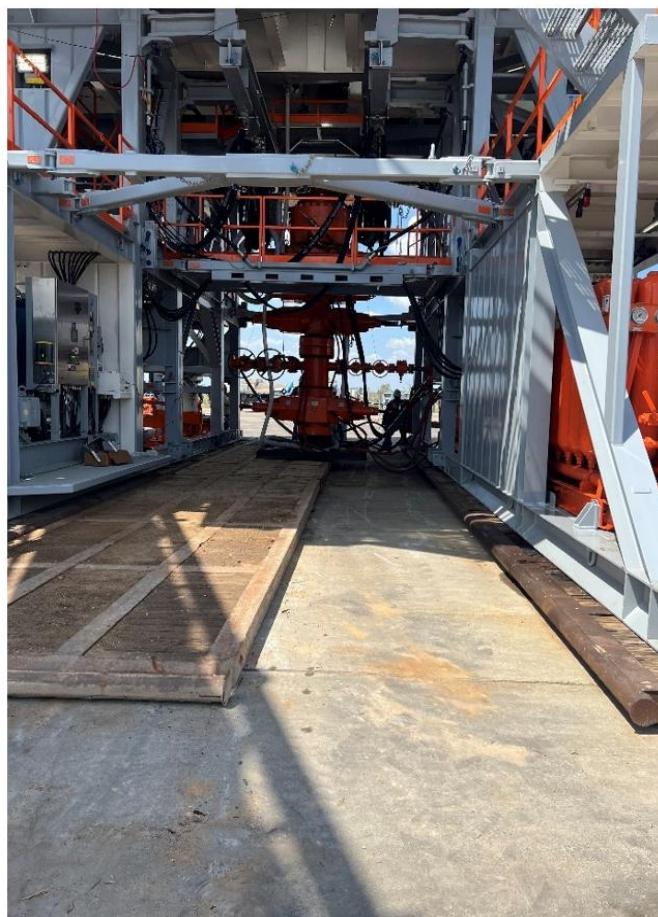
Figures 1 & 2: BOP winch system picture with walking capabilities.
