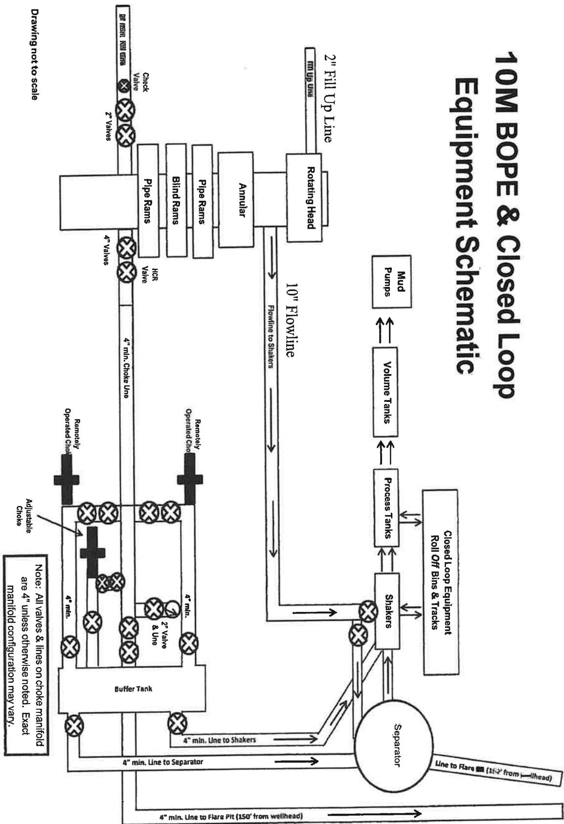
Note: All valves & lines on choke manifold
