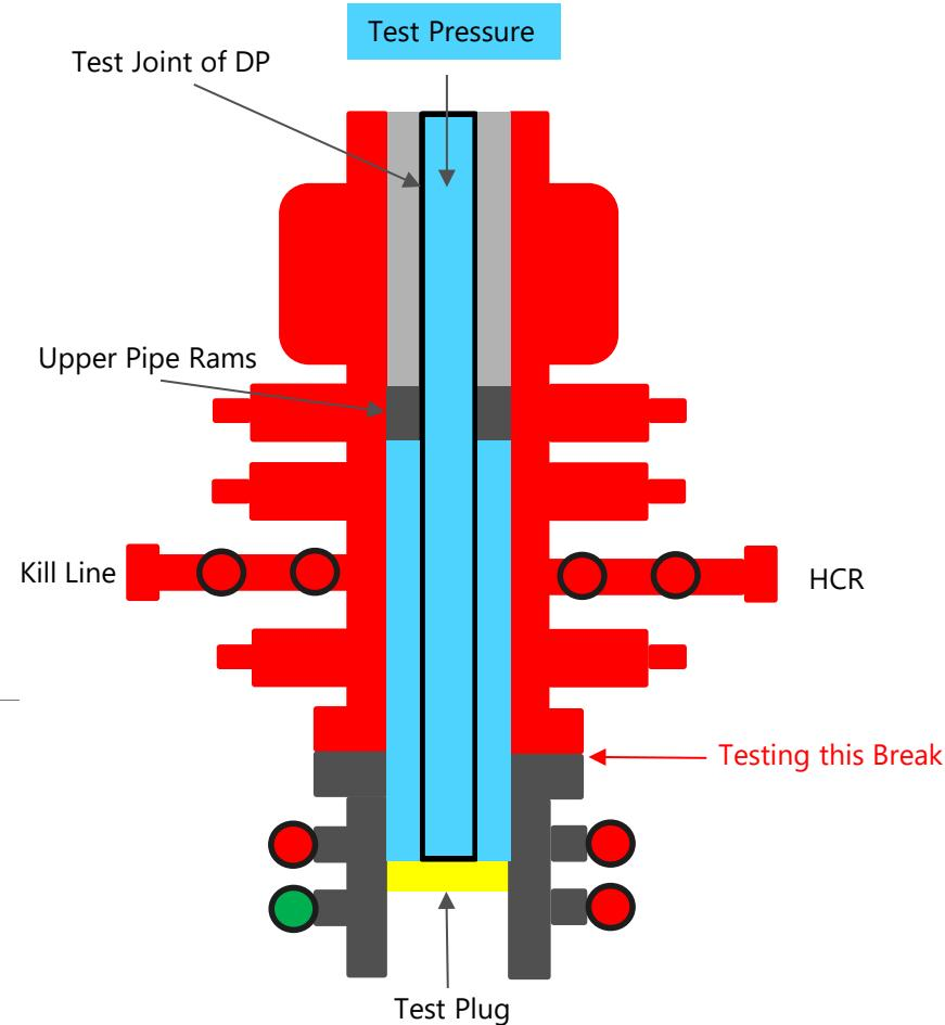
Devon requests offline BOPE testing for the following components: Upper Rams, Blind Rams, Kill Valves, Choke Valves, and Annular
