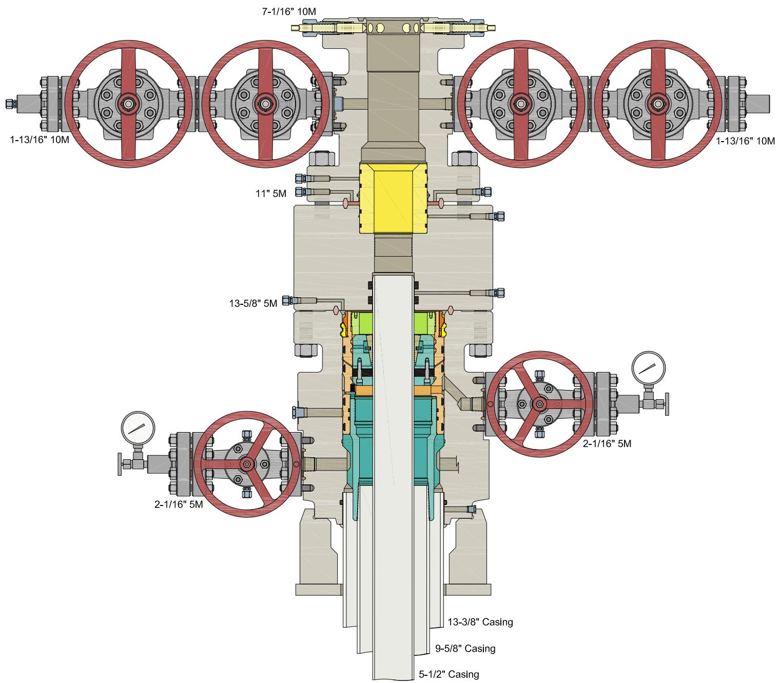
A multibowl wellhead may be used. The BOP will be tested per 43 CFR 3172 after installation on the surface casing which will cover testing requirements for a maximum of 30 days. If any seal subject to test pressure is broken the system must be tested.
