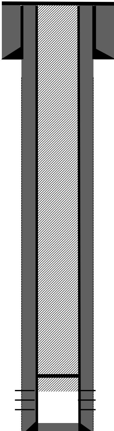
**8-5/8" 24#, J-55 casing @ 129': Hole size - 12-1/4"**Cemented w/ 95 sks, class B neat w/2% CaCl2 w/ 1/4# celloflake/sx.
