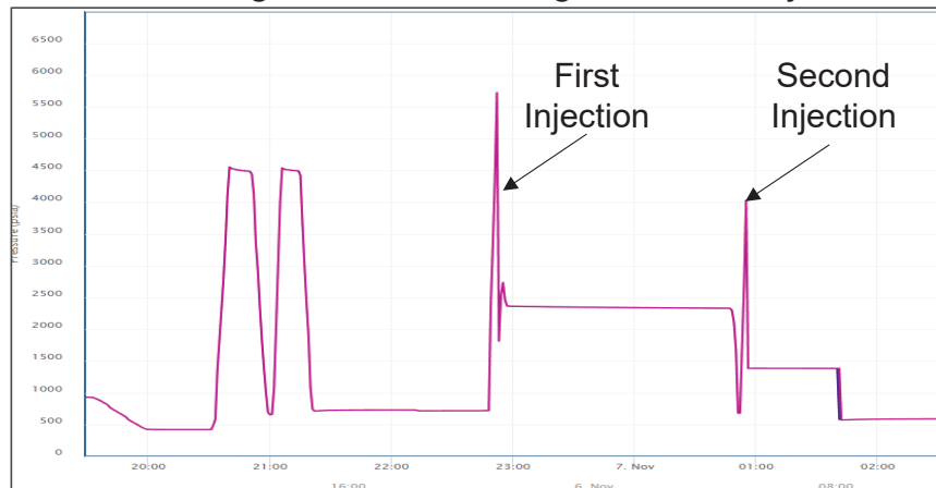
Surface Gauge Pressure during 1st & 2nd Injections
