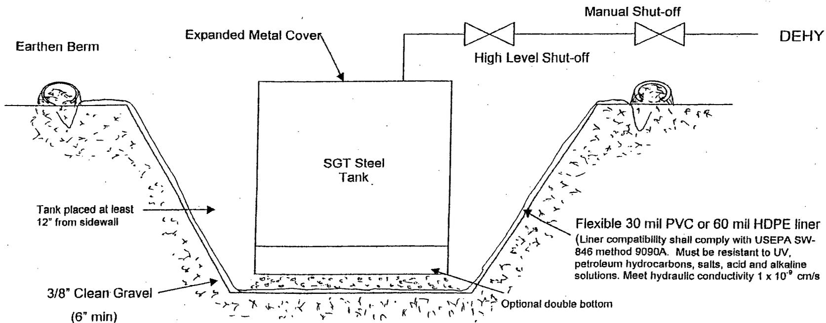
**Note:** Foundation shall be free of rocks and debris and otherwise made level. Liner is anchored at ground surface - min 12 in trench. Installation allows for fluid collection point and visible inspection of exposed liner. Shut-off system designed to maintain 28" freeboard. Installation location should meet siting criteria or be approved by NMOCD.
