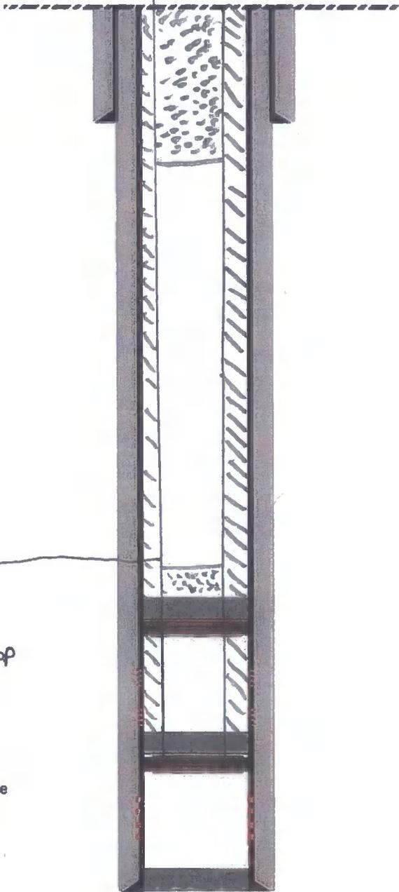
4.5 Set from 1800 to surface Cemented to surface
