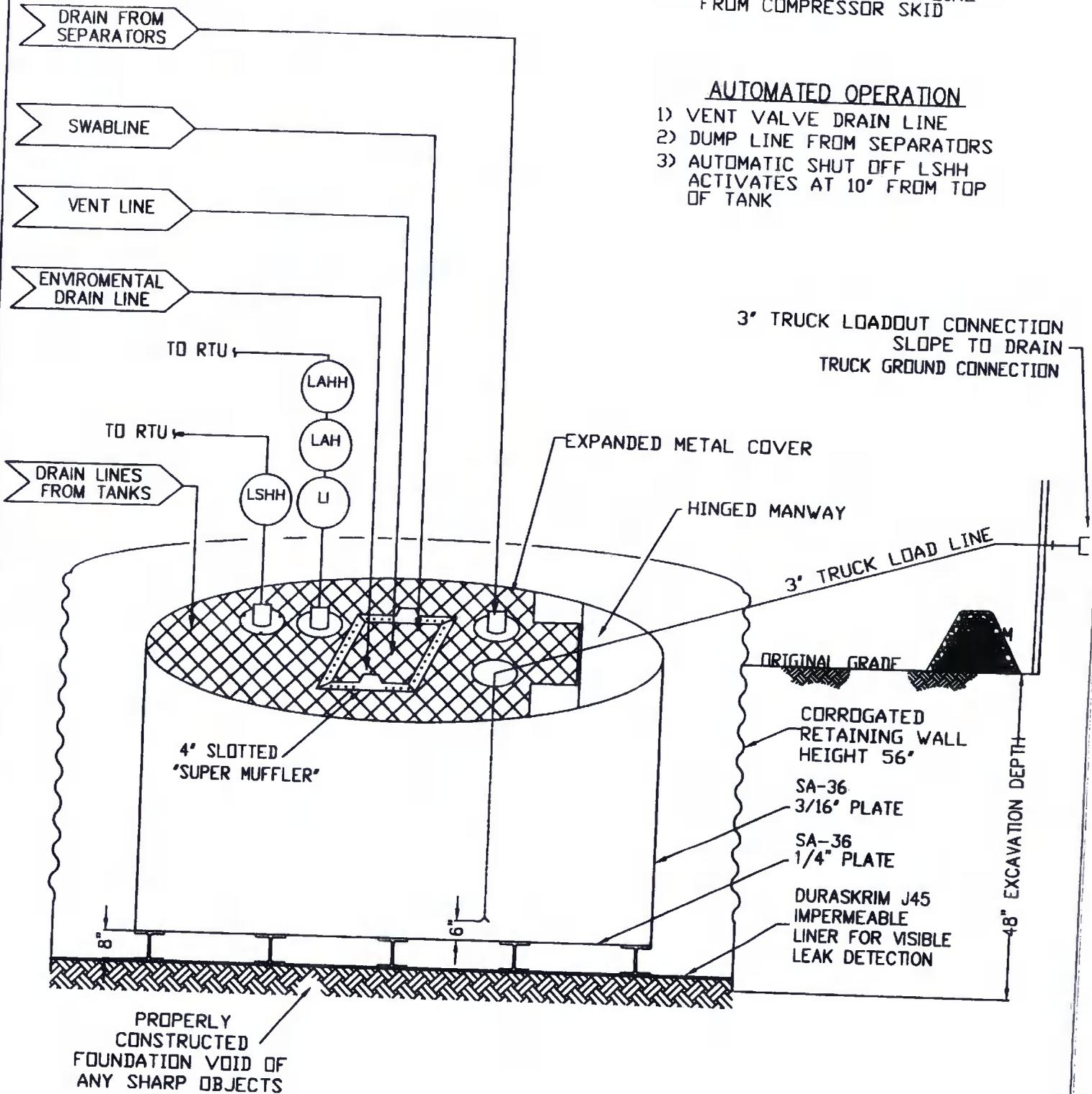
3" TRUCK LOADOUT CONNECTION
