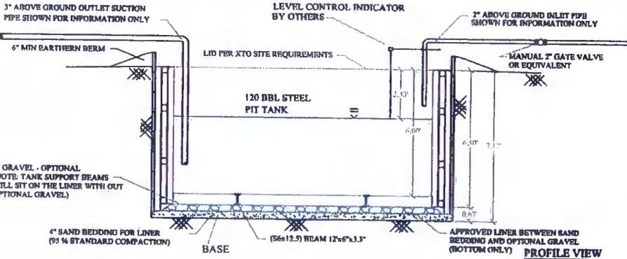
**NOTE: PROVED 6" MIN. EARTHEN BERM AROUND FIT CONTAINMENT TO KEEP SURFACE RUNOFF FROM ENTERING FIT.**
