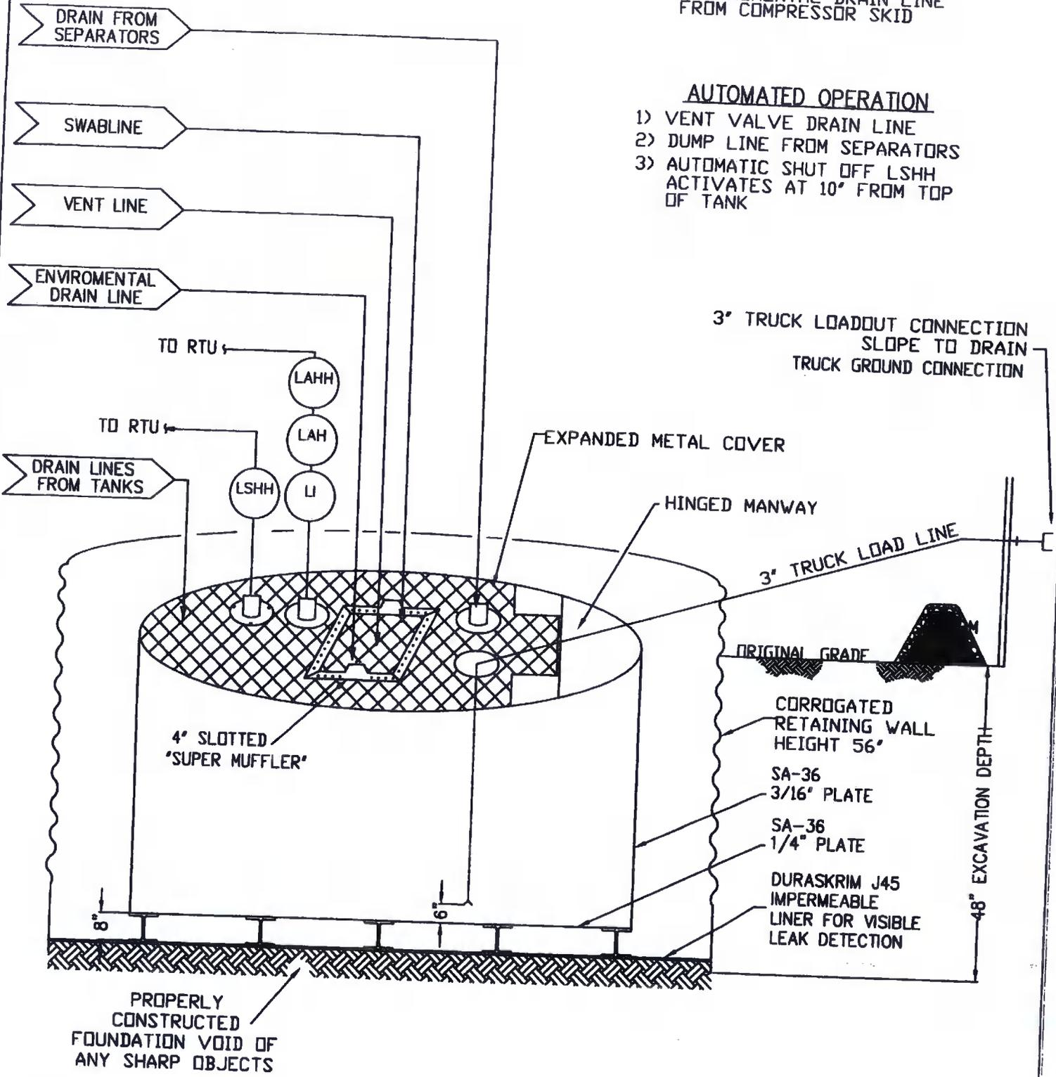
3" TRUCK LOADOUT CONNECTION
