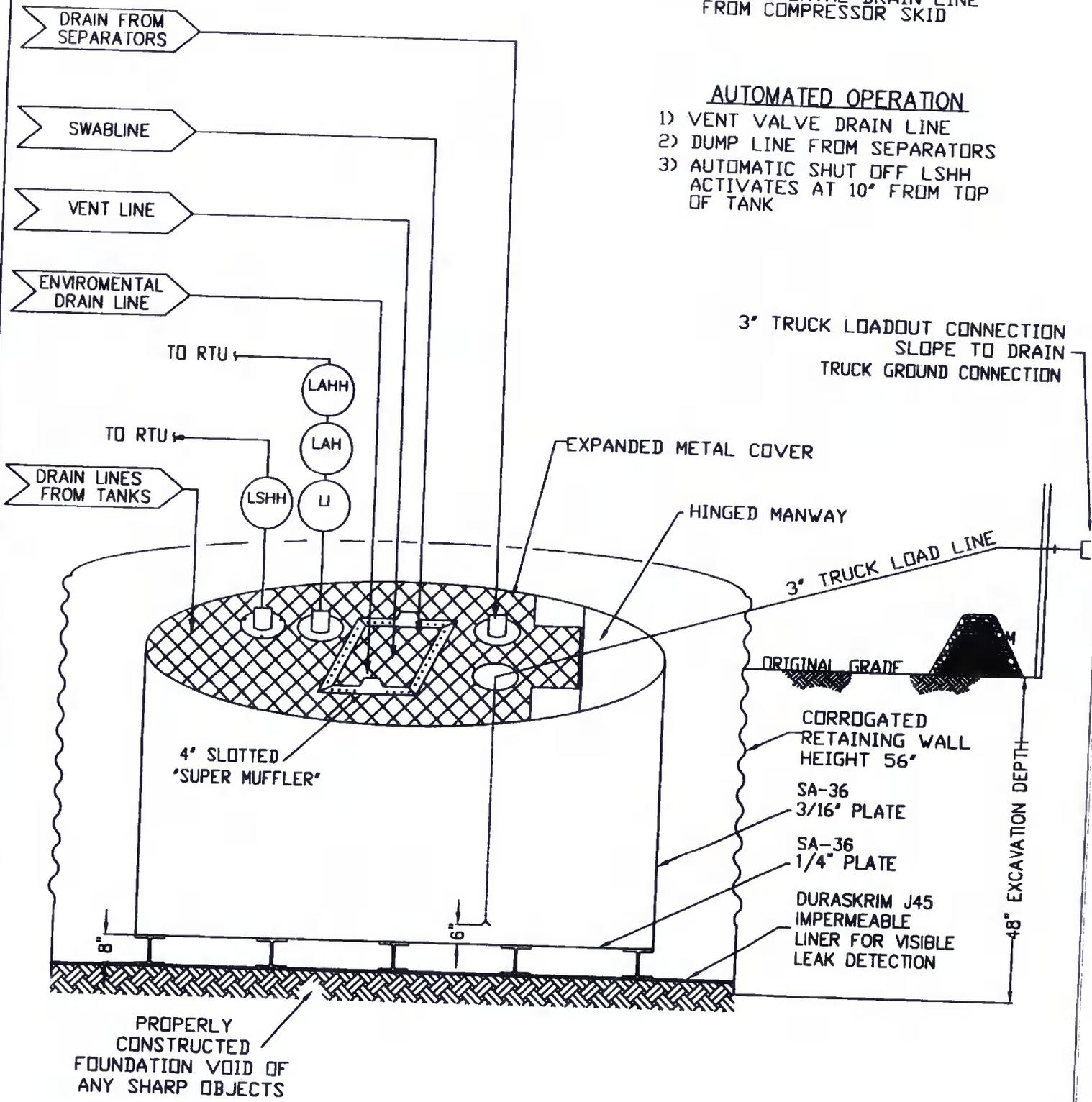
3" TRUCK LOADOUT CONNECTION
