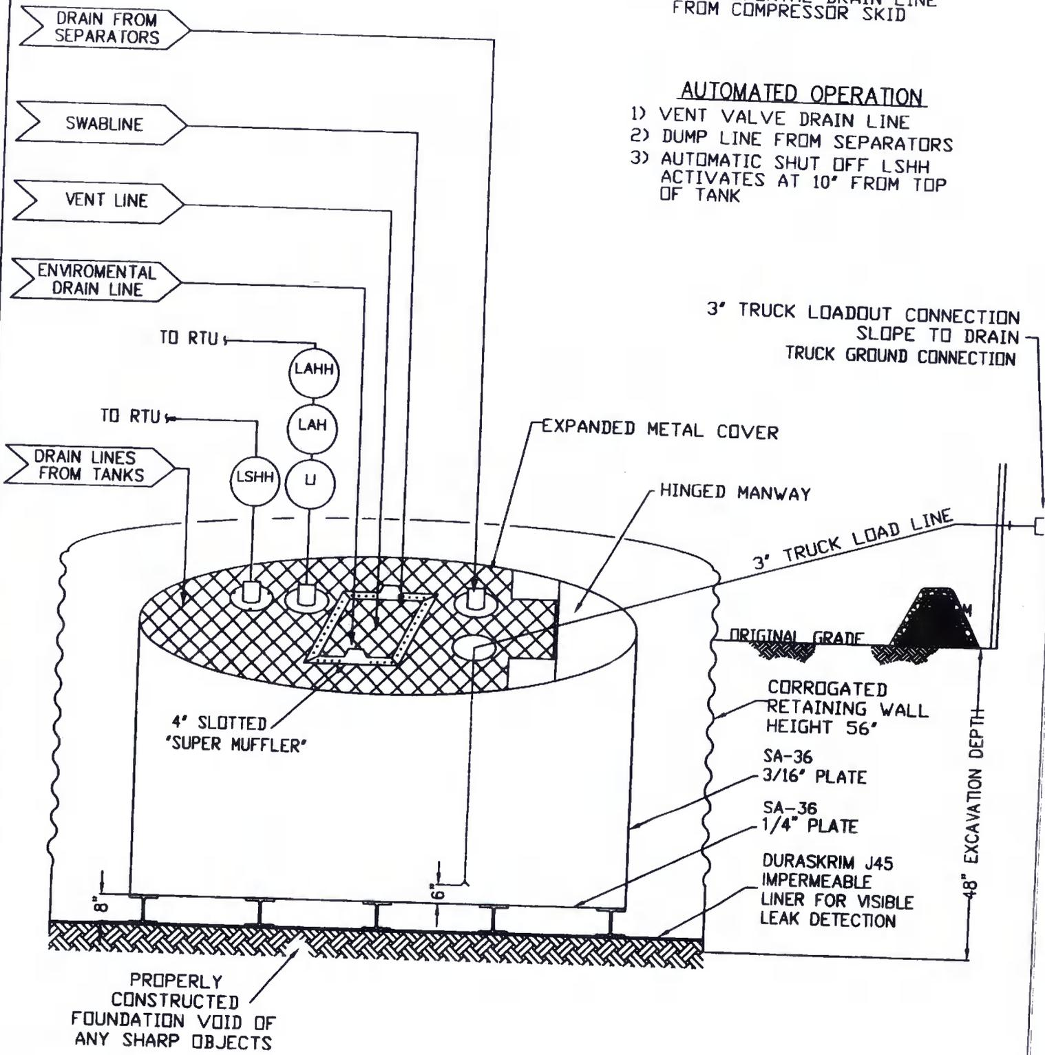
3" TRUCK LOADOUT CONNECTION
