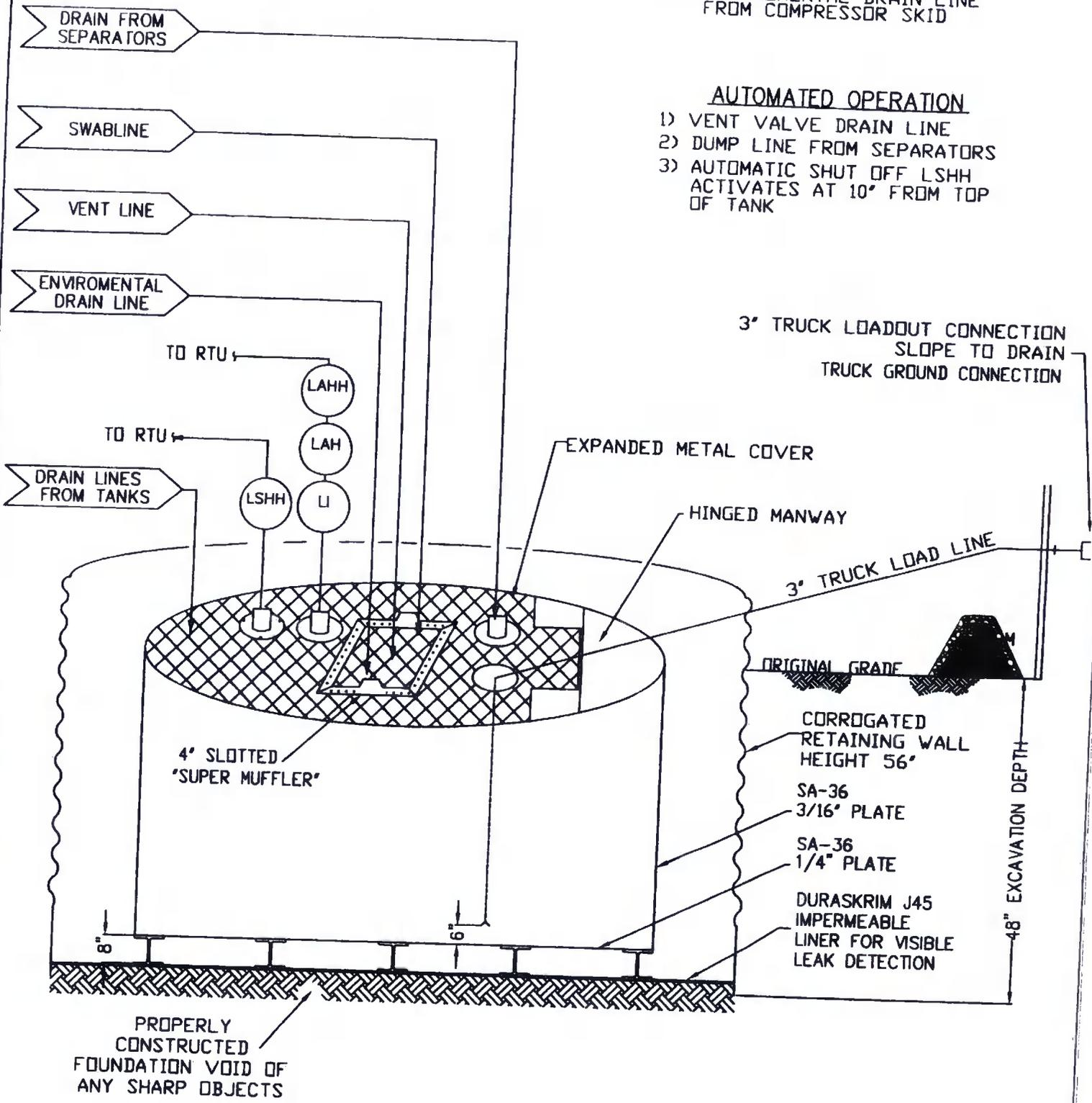
3" TRUCK LOADOUT CONNECTION
