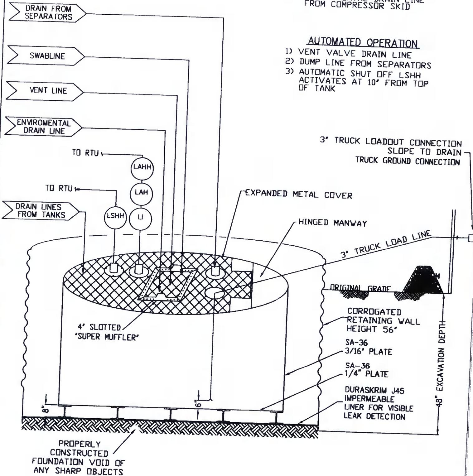
3" TRUCK LOADOUT CONNECTION
