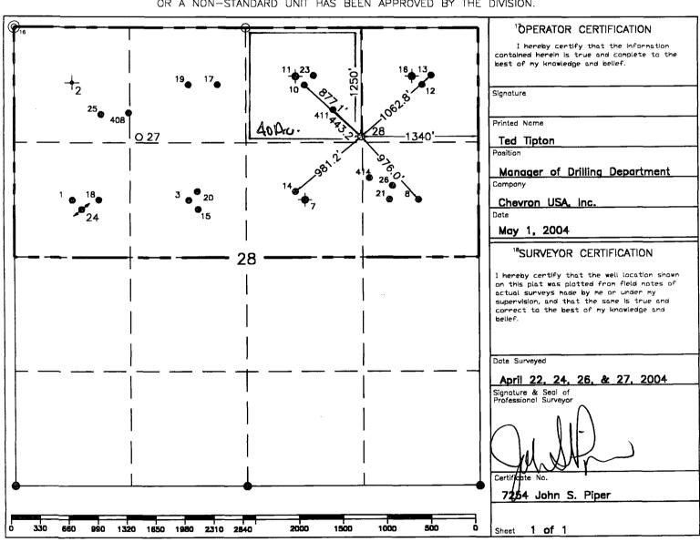
= Injection Well 💠 = Water Supply Well 💠 = Plugged & Abandon Well O = Staked Location ● = Producing Well
