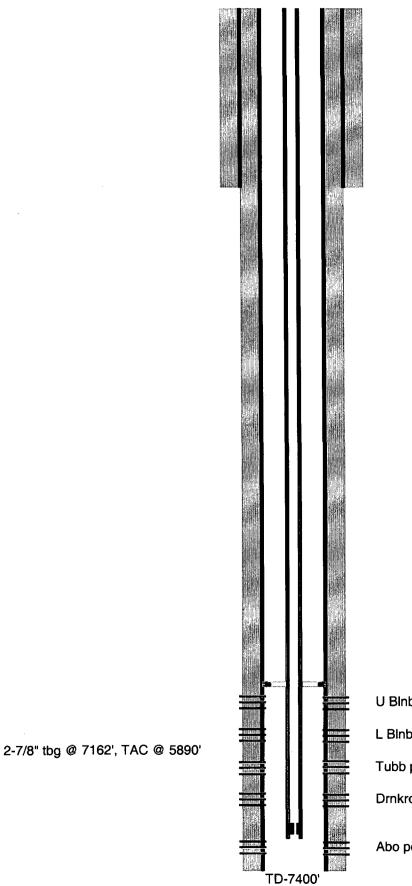
12-1/4" hole @ 1500' 8-5/8" csg @ 1500' w/ 735sx-TOC-Surf-Circ
