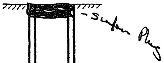
10 <sup>3</sup>/<sub>4</sub> " casing set at 303 ' with 165 sx of Inor cemen
