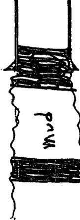
7 <sup>7</sup>/<sub>8</sub> " casing set at 3100 ' with 750 sx of C ceme
