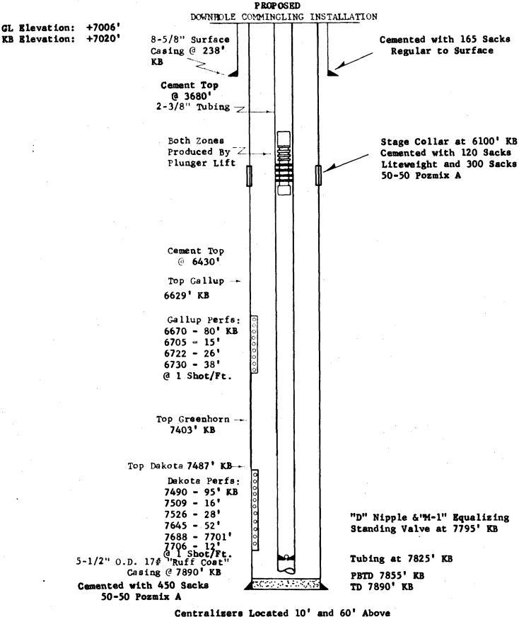
Centralizers Located 10' and 60' Above Casing Setting Depth and 90' Thereafter
