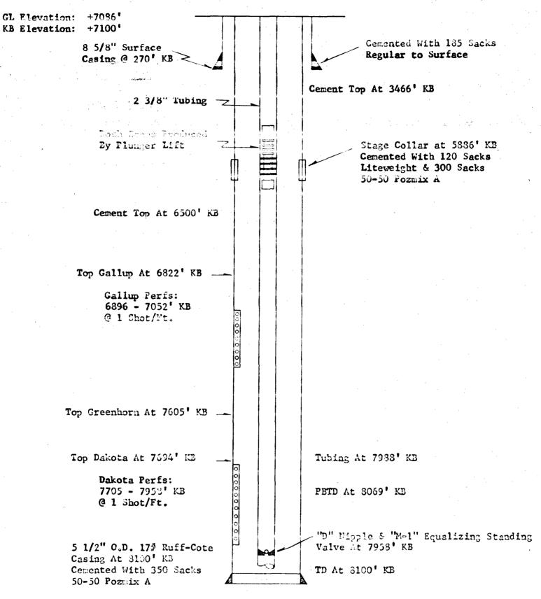
Centralizers Located 10' & 60' Above Casing Setting Depth and 90' Thereafter to 6770' KB; Also One Centralizer 30' Above and 30' Below Stage Collar.
