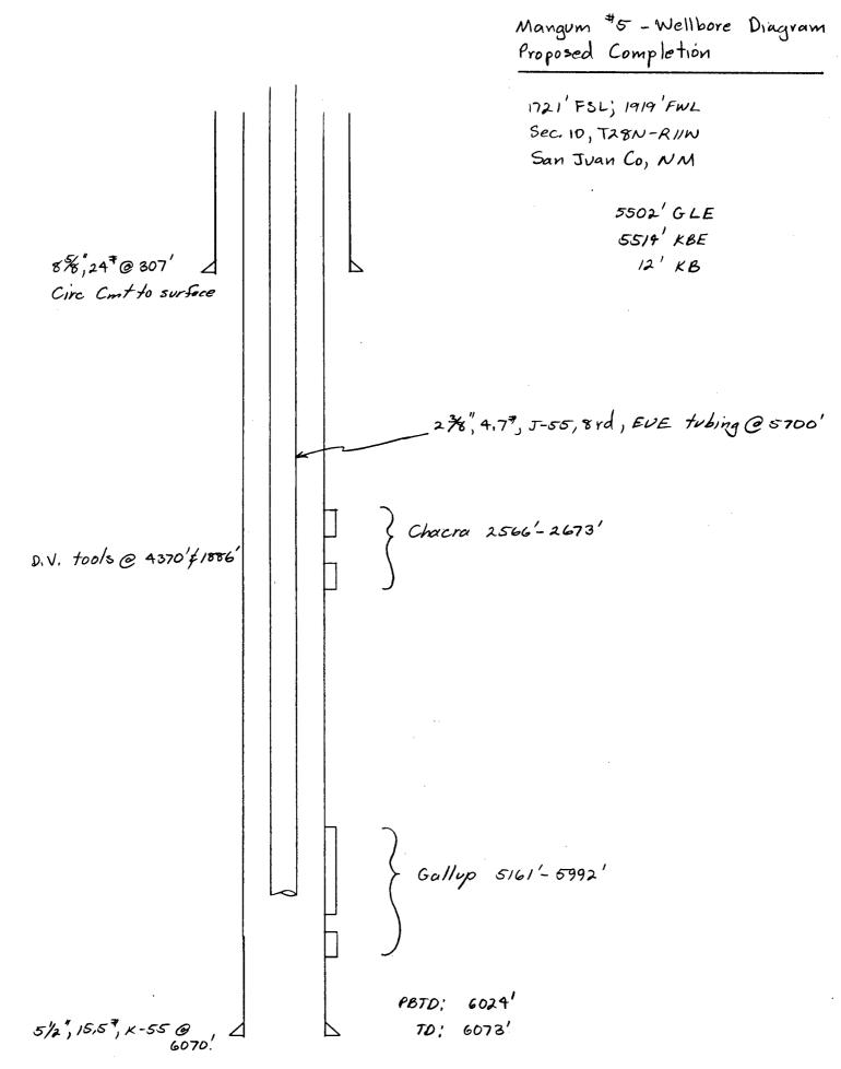
1stage: Cmt w/ 640 ft 3 50/50 POZ w/ 290 gel, .6 % FLA, Y4 Flocele, 10 +30/11/5K: 2nd stage: Cmt w/ 1280 ft 3 65/35 POZ w/ 6% gel, 10 + Gils/sk: Tail w/ 100 sx cl'B" w/ 2% GaC/2 3rd stage: Cmt w/ 1148 ft 3 65/35 POZ w/ 12% gel. 12 1/2 + Gils/sk: circ to surface
