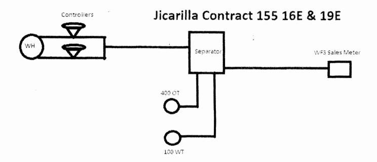
Testing Procedure: For testing/ellocation purposes, the DK will be shut off via the controller for 24 hrs once a month to test the MV production.
