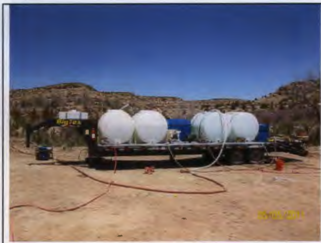
2.) View of the ISCO pump trailer.
