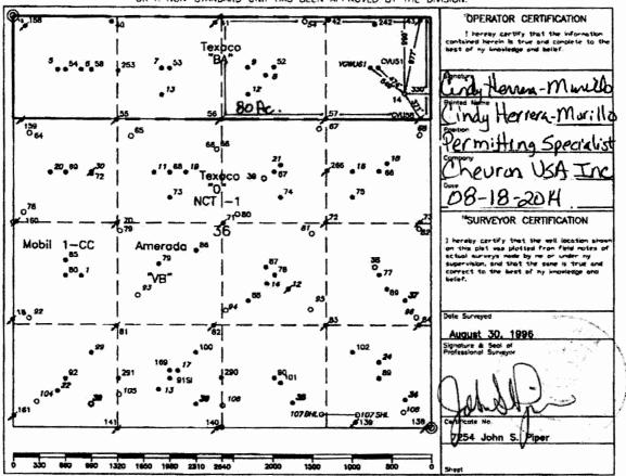
Staked Location • = Producing Well = Injection Well - Water Supply Well - Plugged & Abandon Well (5) = Found Section Corner, 2 or 3" Iron Pipe & GLO B.C. o = Found /4 Section Corner, 1" Iron Pipe & GLO B.C.
