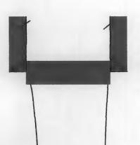
Cut & pulled 570' of 8 5/8" casing
