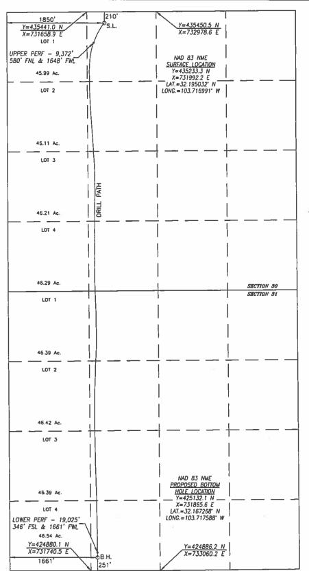
BOREPATH SHOWN HEREON IS BASED ON DIRECTIONAL SURVEY REPORT PROVIDED BY COG FOR THE WINDWARD FEDERAL #7H SUPPLIED TO HARCROW SURVEYING, LLC ON 9/27/17.
