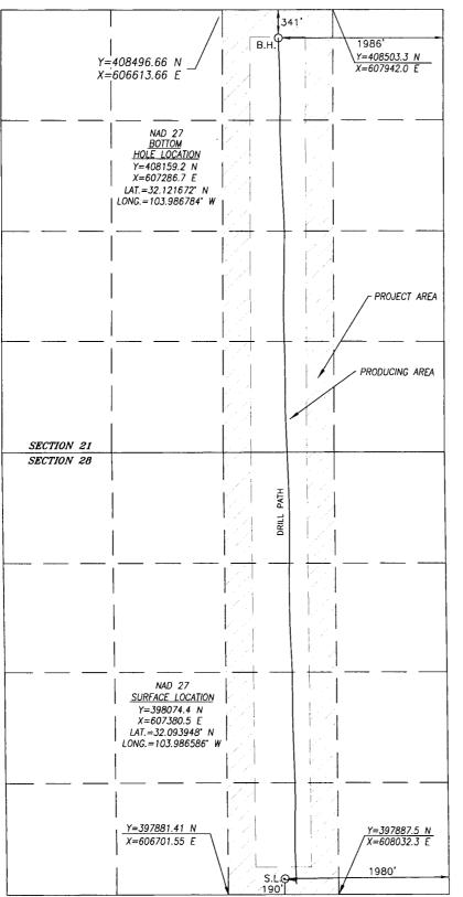
BOREPATH SHOWN HEREON IS BASED ON A DIRECTIONAL SURVEY REPORT PROVIDED BY COG OPERATING, LLC FOR THE ADMIRAL FEDERAL COM #2H ON MAY 27, 2016.
