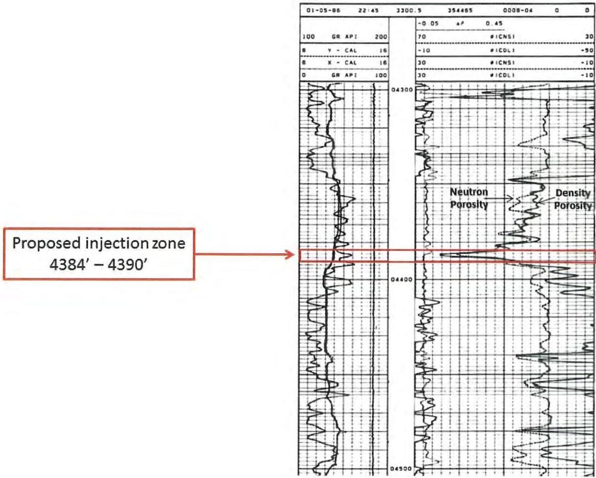
Figure 3. Well log taken from the E-K Queen Unit #212 well illustrating the proposed injection zone in a red box. The injection zone is characterized by an extremely high porosity bed and is confined on either side by about 100' of low porosity beds of limestone, dolomite, anhydrite, etc.
